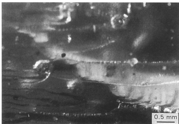
Figure 3 Cleavage step formation and production of elongated particle resulting from fracture plane (moving from left to right) meeting pore.
